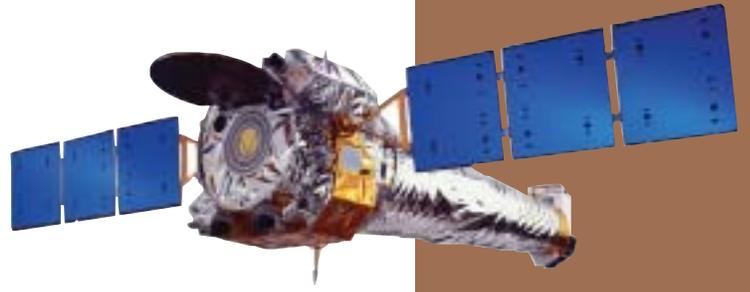
*The Chandra X-ray telescope was designed to measure X-rays from high-energy sources, such as exploding stars or black holes. Built in cooperation with NASA, it represents the largest, most successful externally funded science project in Smithsonian history.*
