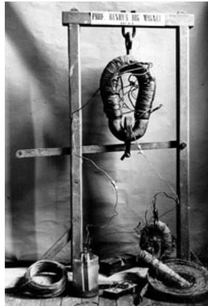
Some of Henry's experimental apparatus, including magnets, a battery, relay switches, and insulated coils. Photo by R. H. Rose. Princeton University physics department.
