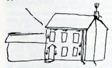
door being under the 1st window. There is a wooden gutter which runs horrizontally along the front of the house under the eaves and at the nor<west>east side this is furnished with a tin pipe of about <4>3 inches indiameter connecting it with the ground. Both the gutter and the pipe
