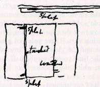
below also on the opposite upright of the frame near the lower hing[e] of the shutter the casing was marked. The gutter was split where the lightning passed down to the window. It made its appearance principally where the nails were inserted. In some case the discharge appeared merely to have touched the *<part>* wood and gouged out a groove of about the 8<sup>th</sup> of an inch
