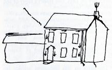
ney would give it.<sup>5</sup> It is made of round iron 3/8th of an inch in diameter and in 5 pieces joined by hook and eye joint. It is terminated above by 3 points which are very blunt but do not exhibit signs of fusion and at the lower end its connection with the earth is very imperfect—it appears to be merely stuck into the ground to the depth of perhaps 2 or three feet. It rises to the hight of about [...]<sup>6</sup> feet above the roof
