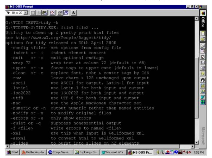
A typical Tidy user command is: C:\migration\tidy \*.htm -f errs.txt This command will list all (-e) errors on the screen and save them in the text file. The migration can be initiated with the following line: Tidy -as xml -clean filename.html > filename.xhtml
