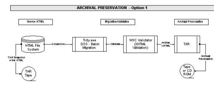
This implementation option calls for the combination of Tide.exe (DOS batch mode) to migrate HTML pages to XHTML and direct access to the W3C Validation Service to ensure that the XHTML pages comply with the W3C standard.
